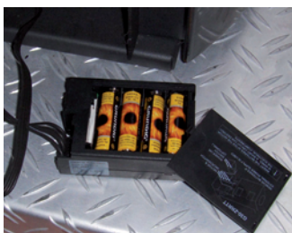
Replacing the batteries of the receiver
