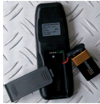
Replacing the batteries in the remote control
