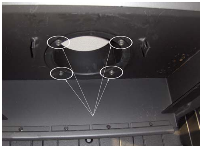
Illustration 1 Remove the pipe collar from the hearth
